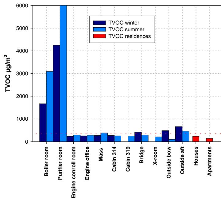
Figure 3. Concentration of TVOC in the various spaces onboard the icebreaker Oden. The information from Swedish residences is added for comparison. The dashed line represents the hygienically safe level of  $300 \mu\text{g}/\text{m}^3$  as specified by the Federal Environment Agency of Germany (UBA).
