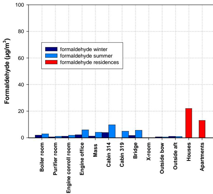
Figure 2. Concentration of formaldehyde in the various spaces onboard the icebreaker Oden. The information from Swedish residences is added for comparison.
