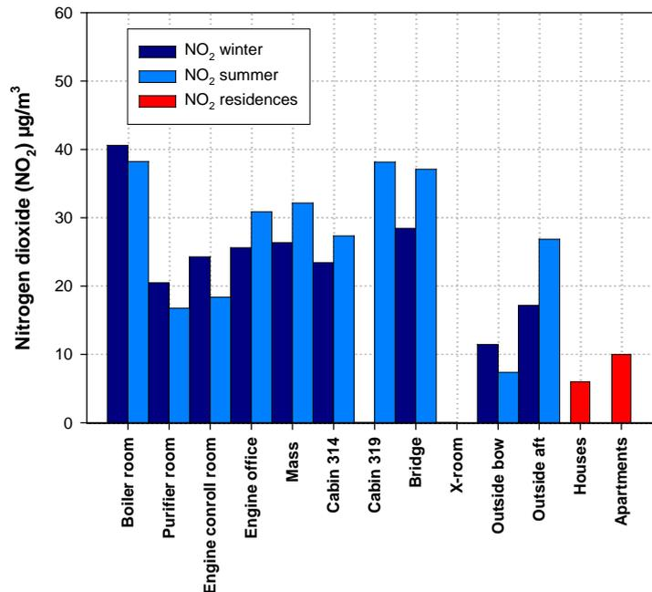
Figure 1. Concentration of NO<sub>2</sub> in the various spaces onboard the icebreaker Oden. The information from Swedish residences is added for comparison.
