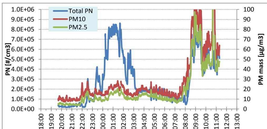
Figure 4. Particle concentration as a function of the operation mode of the main engines (ME): total number concentration (Total PN) and PM<sub>10</sub> and PM<sub>2.5</sub> mass concentrations as continuously measured by optical particle counter. 8 – 22 ME off, 22 – 03 ME on, 03 – 7:45 ME off 7:45 – 11:30 ME on.
