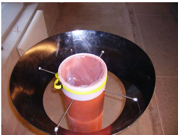
Figure 4. The wind shield (60° funnel) mounted on the bulk collector. The disposable plastic bag is held in place by a thin polyethylene ring.
