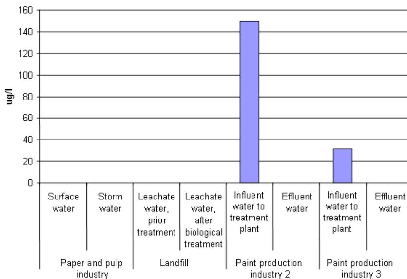
Figur 3. IPBC concentrations (ug/l) in influent and effluent water at treatment plants at paint industries, paper and pulp industry and from a landfill (recycling company).
