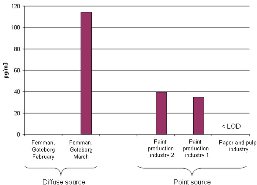
Figur 2. Concentrations of IPBC (pg/m<sup>3</sup>) in air from a diffuse urban area and from point sources, i.e. paint industry and paper and pulp industry.
