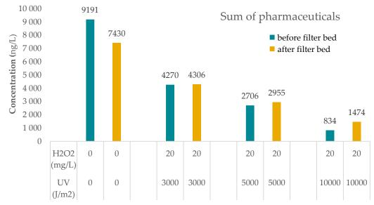
Figure 6. Effect of filter bed on pharmaceutical concentrations.
