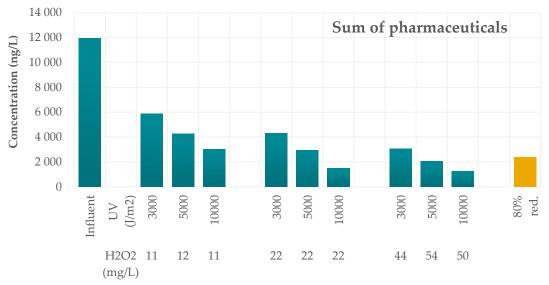
Figure 3. Sum of pharmaceutical concentrations analyses in the pilot tests.
