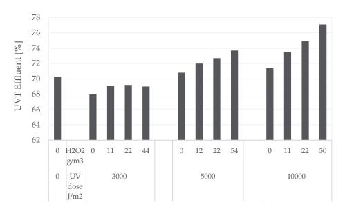
Figure 2. Transmittance of the treated water after the UV/H2O2 treatment for the various dose combinations.
