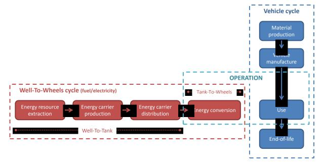
Both vehicle life cycle and fuel/electricity life cycle were included in the GaBi models. Vehicle life cycle comprises of material and vehicle production, use (including maintenance) and end-of-life phases (Figure A3 in blue). Operation energy requirements (fuel/electricity, Figure A3 in red), maintenance and end-of-life were modelled using Ecoinvent datasets of passenger and city cars. Those datasets are based on the performance of vehicles of comparable size, mass, and power.
