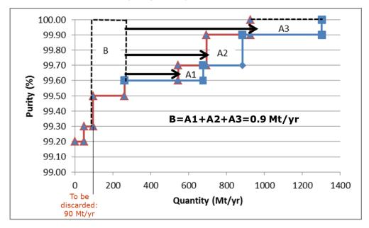
Figure 17: Optimum mixing of steel scrap in the material pinch analysis of Ekvall et al. (2014). The excess purity is given by the area A1+A2+A3.
