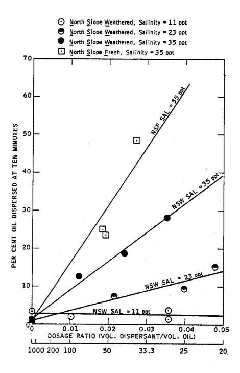
**Figure 2.** Water's salinity is directly proportional to how much a certain oil can disperse. The figure illustrates the oil North Slope at various salinities. (Lehtinen, 1981).
