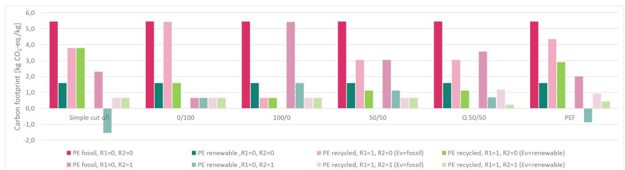
Figure 3.3: Carbon footprint results from the Essity case study on plastic packaging alternatives with application of selected approaches to allocation at recycling and with biogenic carbon removals attributed to primary production (cultivation).
