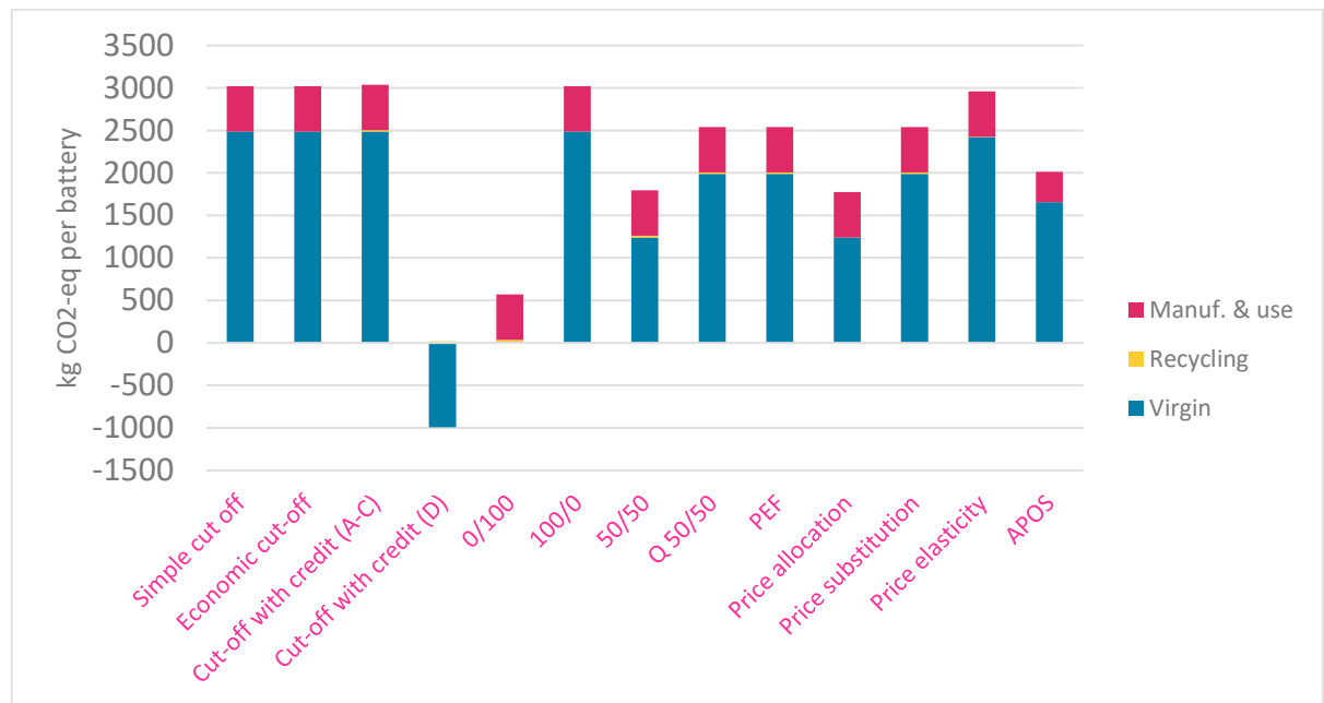
Figure 9.1: CO 2 eq. results from an LCA of a battery in an electric Volvo bus, which, after use is reused for another purpose.
