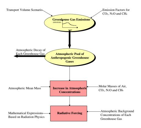
Figure 2.1 Schematic view of the model used to calculate radiative forcing for future Swedish transport scenarios.
