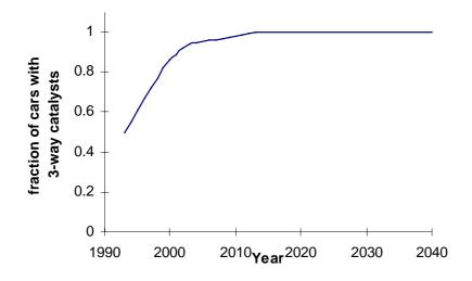
*Figure 6.1 Fraction of passenger cars with 3-way catalysts from 1990 to 2040 (Brandel & Sjödin, 1995).*
