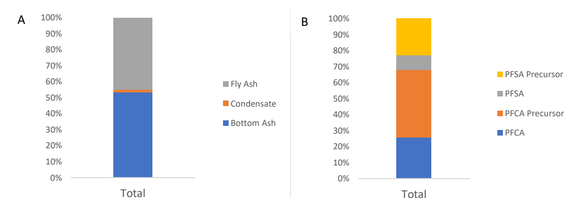
Figure 6. Estimation of PFAS emissions from the Swedish incineration plants: A) Relative contribution from different incineration residuals (bottom ash, fly ash and condensate). B) Relative composition of PFAS classes in the total potential annual emissions of PFAS in the studied Swedish incinerations.
