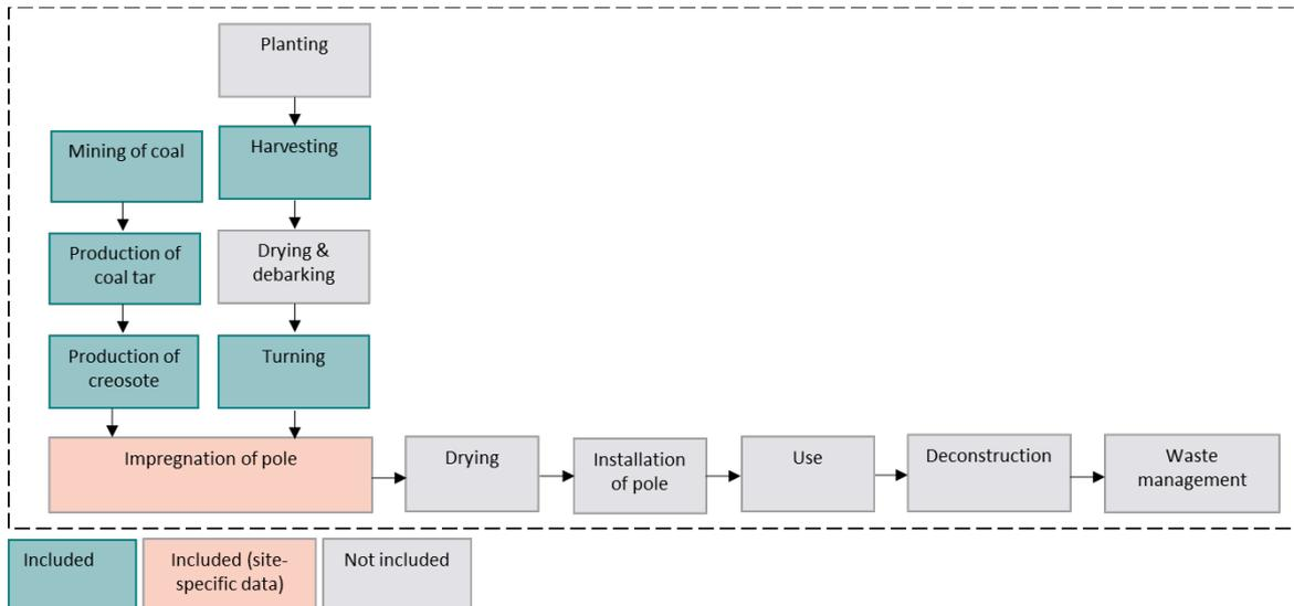
Figure 1: Overview of the life cycle of the wood based pole impregnated with creosote. The green boxes are the processes included in the assessment, the pink boxes are the process with site-specific data and included the assessment, while the grey boxes are the processes not included.
