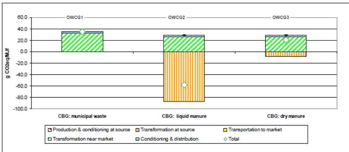
**Figure 2.3** Well-to-wheel GHG balance for compressed biogas pathways (JRC, 2006)
