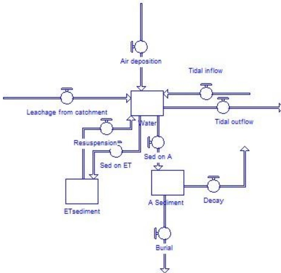
**Figure 2. Outline of the model, where “Water” represents the total volume of the water body of the river delta in Ogoniland. “ET-sediment” represents erosion and transport areas where settling fine matter, by time will be resuspended. “A-sediment” represents accumulation areas with a net deposition of fine matter.**
