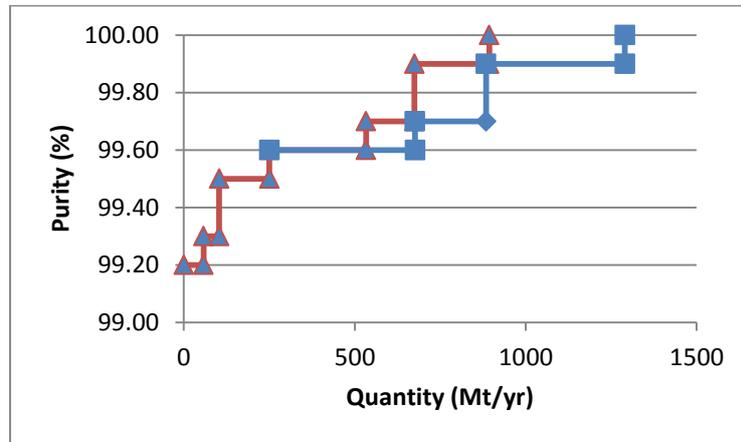
**Figure 5. The two composite curves in the same diagram and with the sink composite curve shifted to the right to identify the pinch point.**
