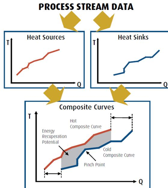
**Figure 2. A principal tool in energy pinch analysis is the graphic representation of composite curves (Natural Resources Canada, 2003).**
