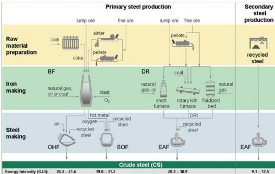
Figure 1. The two steel production routes (World Steel Association, 2011a).
