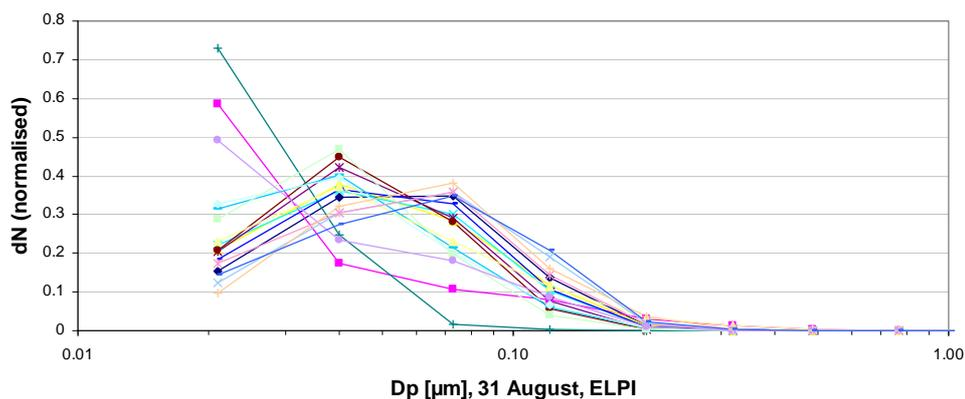
Figure 17 Particle size distributions in vehicle emission plumes obtained by the ELPI on 31 August 2006. Three different classes of size distributions were identified, peaking at  $\leq 0.02 \mu m$ ,  $0.04 \mu m$  and between  $0.04$  and  $0.07 \mu m$ .
