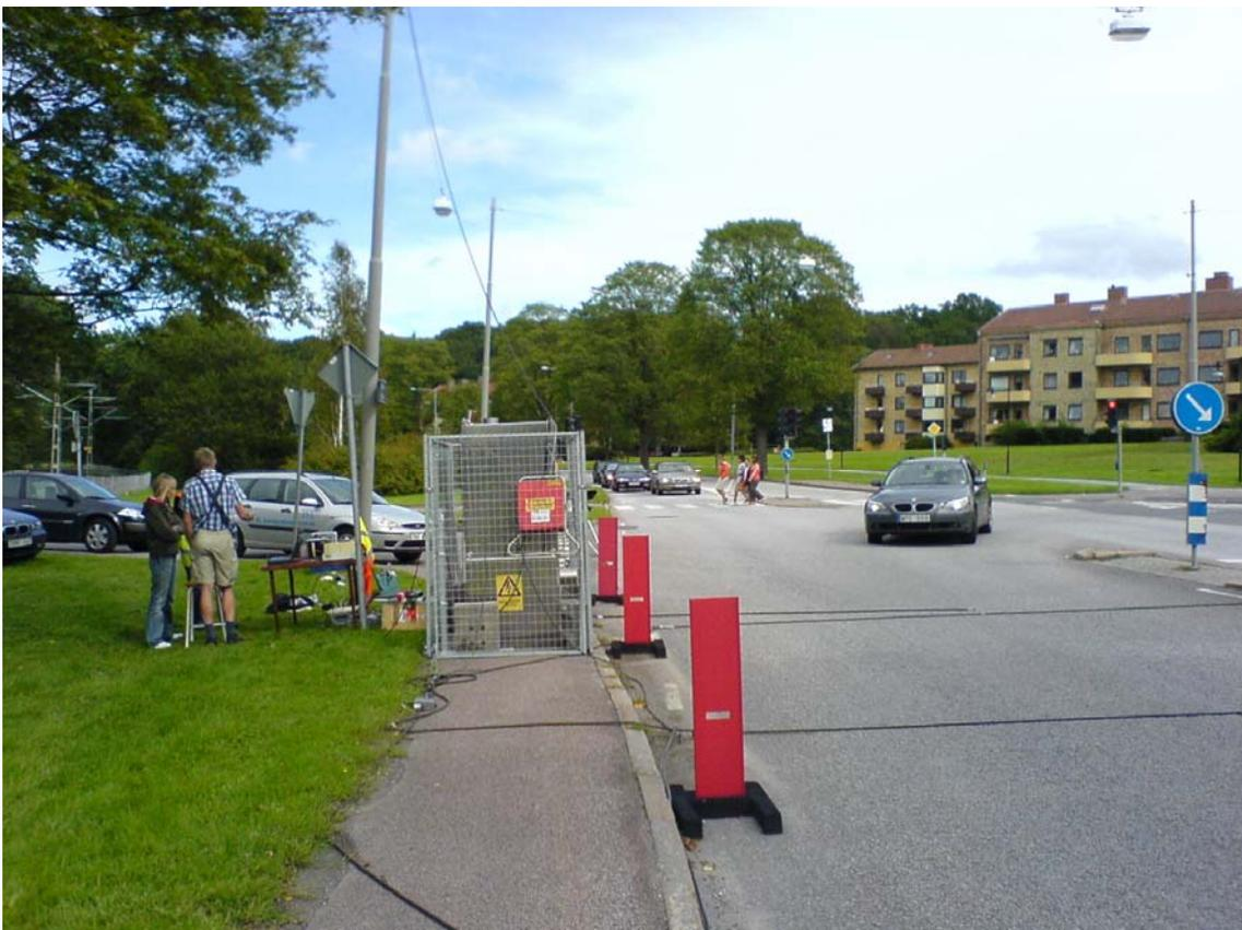
Figure 1 The measurement site with the FEAT instruments in the cabinet. The reflector is on the right side of the road (not seen). The particle instruments are on the table. The particles are sampled with the black tubing that ends in the middle of the lane. The other tubes are for measurements of speed and acceleration. The noise measurement equipment is located behind the photographer (not seen).
