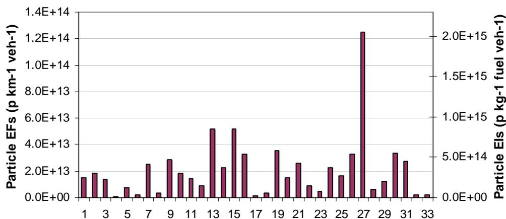
Figure 16. Emission factors for particle emissions from 33 different vehicles.
