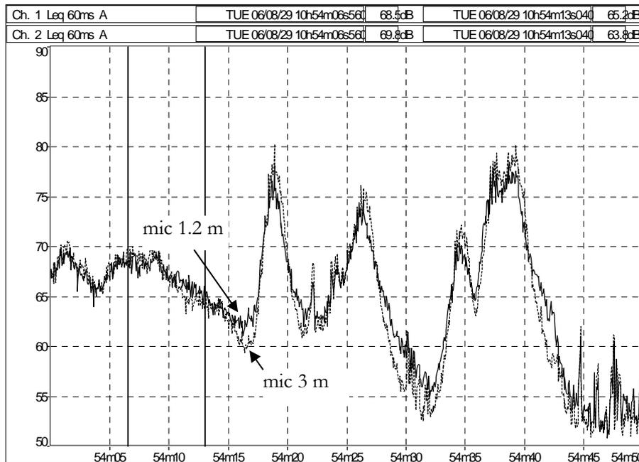
Figure 9 Sound pressure level in a situation where the vehicles are too close. On the axes: x-axis time [s], y-axis sound pressure level [dB re 20  $\mu$ Pa].
