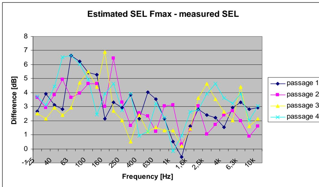
Figure 14 Difference between normalized sound exposure levels estimated from the  $L_{Fmax}$  and the measured  $L_E$ .
