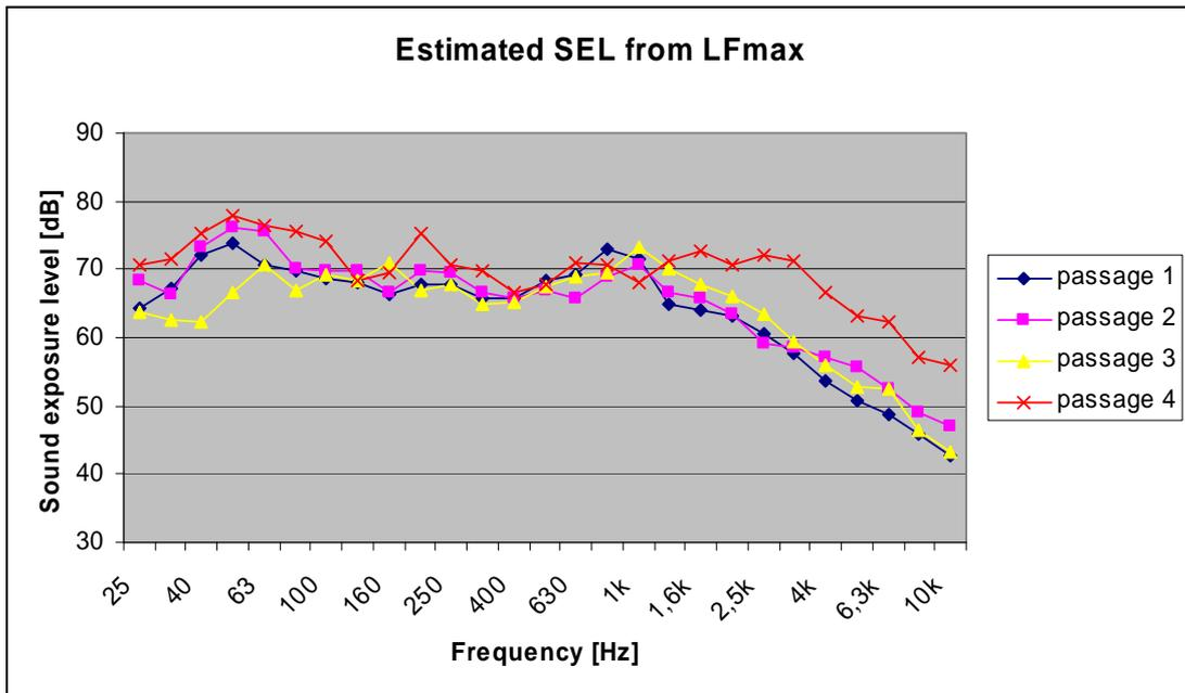
Figure 29 Sound exposure level estimated from the maximum levels of the passages.
