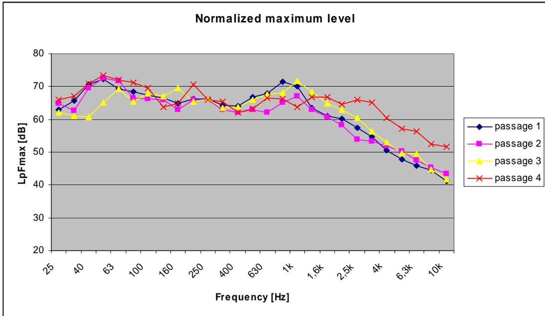
Figure 28 Normalized maximum levels for the vehicle.
