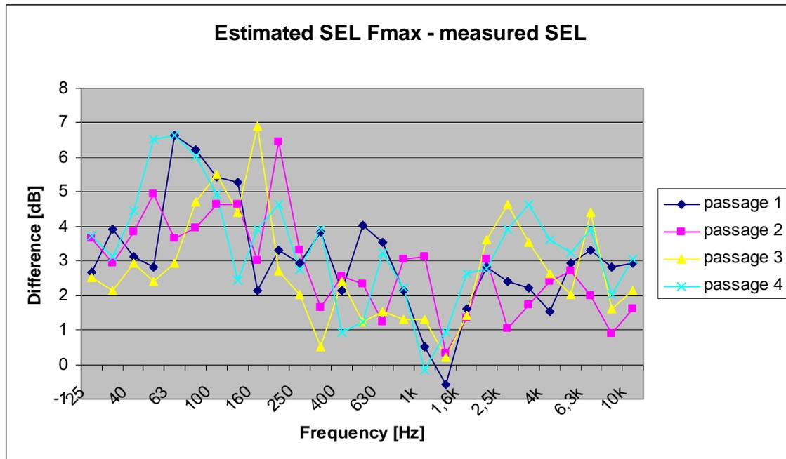
Figure 30 Difference between normalized sound exposure level estimated from the  $L_{Fmax}$  and the measured.
