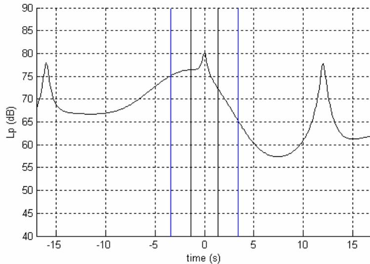
Figure 4 Same vehicles as in Figure 3 but now with an unidentified noise added. Lines for  $\pm 5d$  and  $\pm 2d$  limits are included. As only an  $L_{pFmax}$  value of the pass-by noise is possible to evaluate, the measurement accuracy of this passage is reduced.
