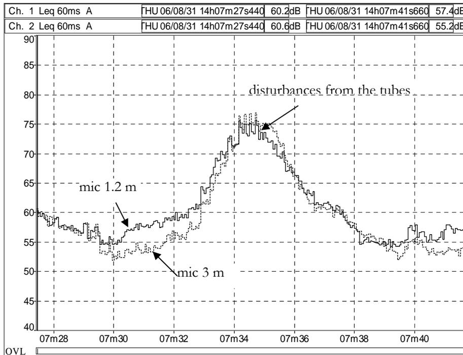
Figure 10 Sound pressure levels when noise from the tubes influences the measurement. The impacts can be seen at the top of the peak in the pass-by. On the axes: x-axis time [s], y-axis sound pressure level [dB re 20  $\mu$ Pa].
