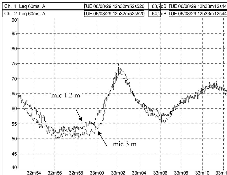
Figure 20 Pass-by of a small passenger car. On the axes: x-axis time [s], y-axis sound pressure level [dB re 20  $\mu$ Pa].
