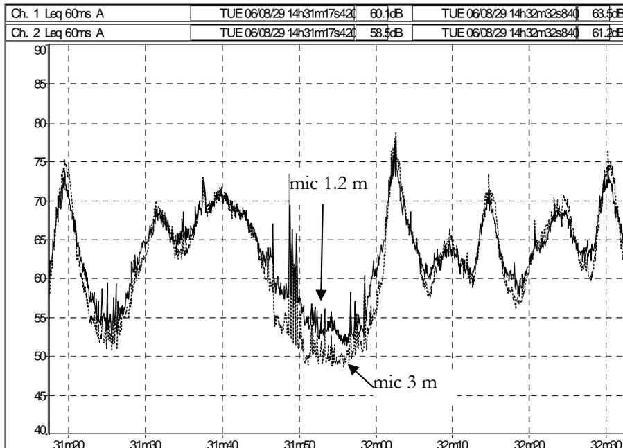
Figure 26 Measurement signal with a relatively high background noise. On the axes: x-axis time [s], y-axis sound pressure level [dB re 20 µPa].
