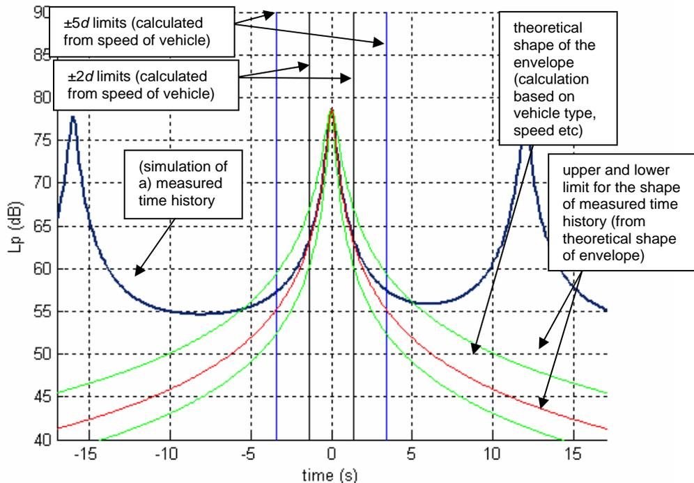
Figure 3 Lines for  $\pm 5d$  and  $\pm 2d$  limits as well as for the shape of the envelope calculated and applied together with the recording. Since the measured time history is between upper and lower limits for the envelope shape not only between the  $\pm 2d$  limit lines but also between the  $\pm 5d$  limit this step in the quality test is passed without deterioration of the accuracy.
