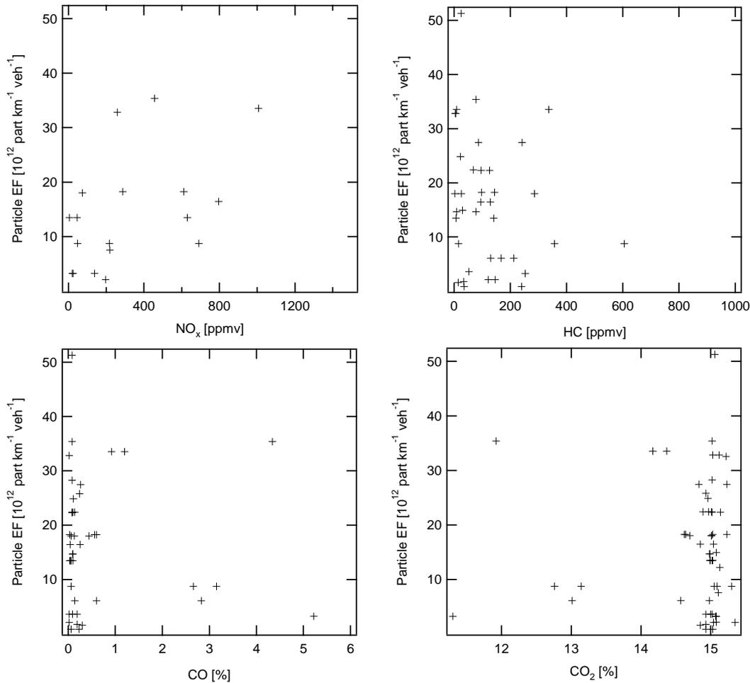
Figure 19: Relationships between particle emissions and trace gas emissions obtained from simultaneous measurements with the particle setup (cp. Sec. 2.3) and the FEAT system. Particle emission factors (EF) are plotted versus the fractions of NO<sub>x</sub>, hydrocarbons, CO and CO<sub>2</sub>, respectively, in the exhaust plumes of passing vehicles. See text for details.
