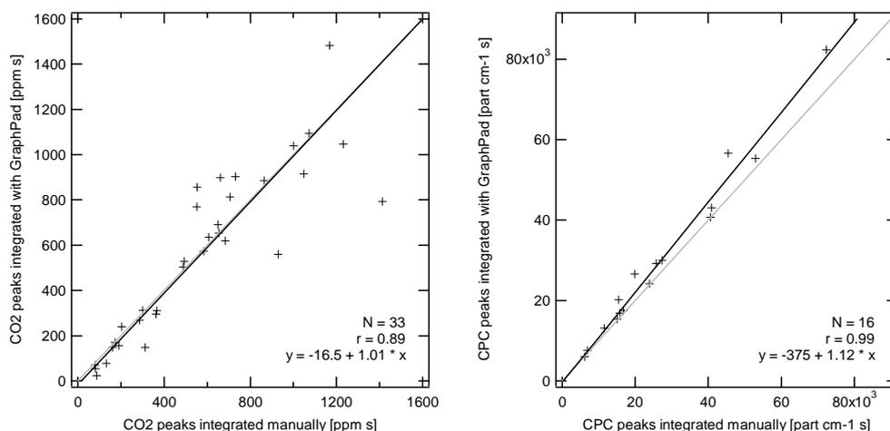
Figure 15 Scatter plots of analytically versus geometrically integrated (left) CO<sub>2</sub> and (right) particle peak areas (measurements of 29 August 2006). The results of an orthogonal linear regression analysis are given within the figures.
