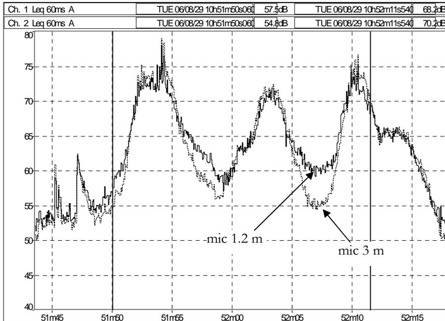
Figure 25 Measured sound pressure levels for two cars passing by at the closest lane and a car in the middle at the opposite lane. On the axes: x-axis time [s], y-axis sound pressure level [dB re 20 µPa].
