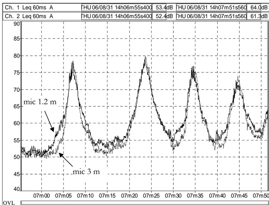
Figure 8 Time record of the sound pressure levels at the two microphone-positions for four vehicles passing by the measurement site. On the axes: x-axis time [s], y-axis sound pressure level [dB re 20  $\mu$ Pa].
