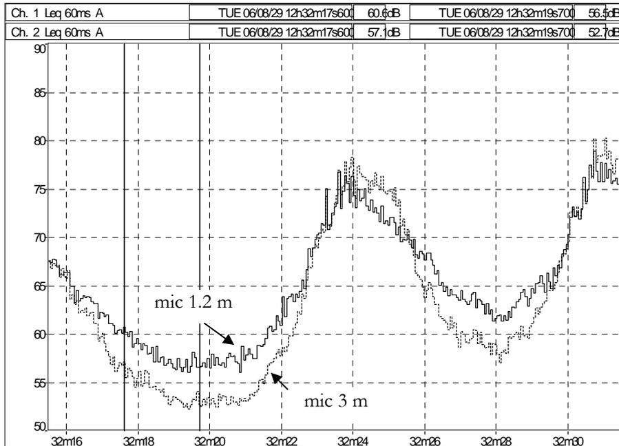
Figure 21 Pass-by of a large passenger car. On the axes: x-axis time [s], y-axis sound pressure level [dB re 20 µPa].
