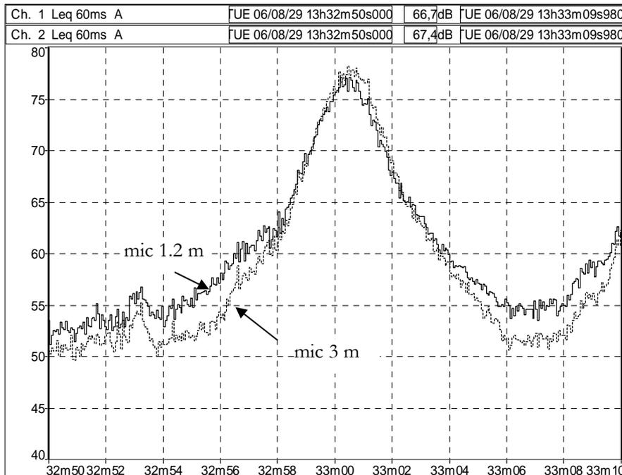
Figure 22 Pass-by of a 2 axle truck. On the axes: x-axis time [s], y-axis sound pressure level [dB re 20 µPa].
