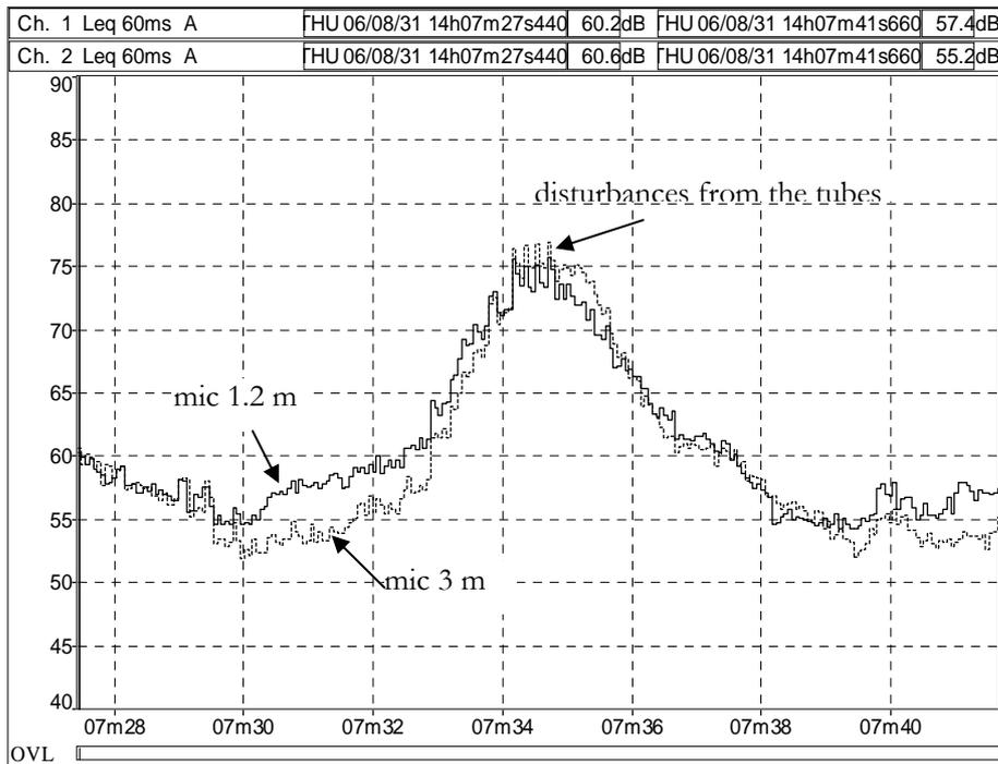
Figure 24 Sound pressure levels when noise from the tubes influences the measurement. The four impacts can be seen at the top of the peak in the pass-by. On the axes: x-axis time [s], y-axis sound pressure level [dB re 20  $\mu$ Pa].
