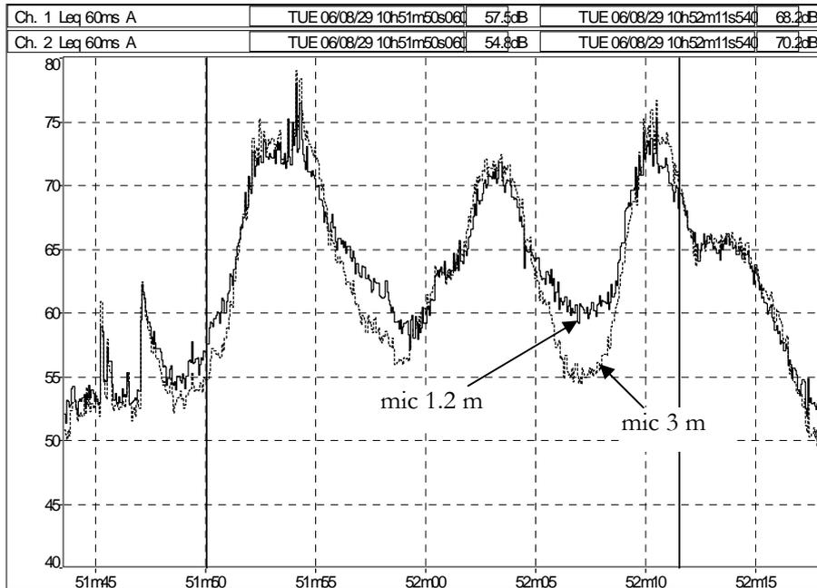
Figure 11 Measured sound pressure levels for two cars passing by at the closest lane and a car in the middle at the opposite lane. On the axes: x-axis time [s], y-axis sound pressure level [dB re 20 µPa].
