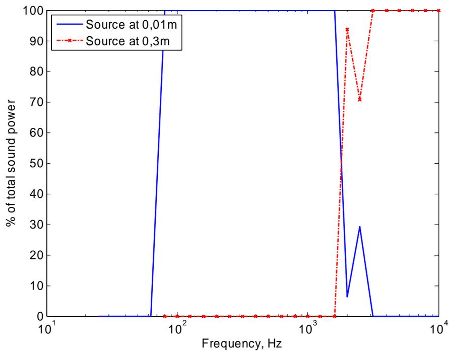
Figure 31 Distribution of sound power between the sources in the source model.
