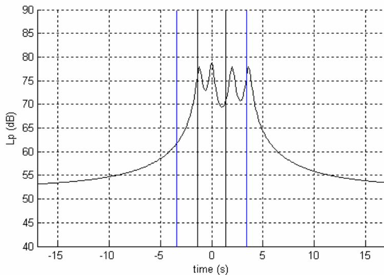
Figure 5 Four vehicles driving in a row rather close to each other. Lines for  $\pm 5d$  and  $\pm 2d$  limits are included. Evaluation of the individual vehicles could only be achieved by means of  $L_{pFmax}$  resulting in reduced accuracy. If all four vehicles belong to the same category  $L_E$  could be calculated for them grouped together.
