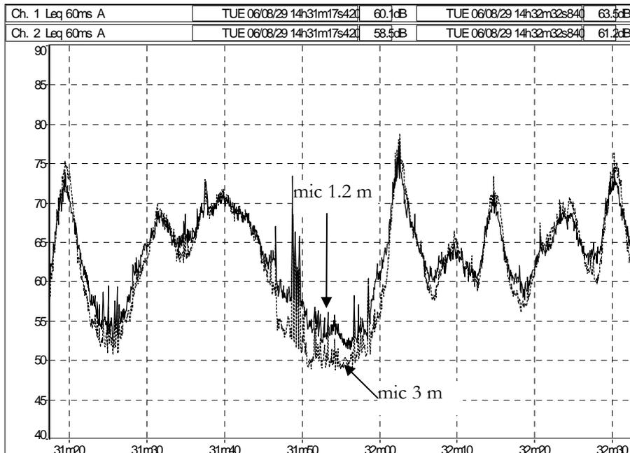
Figure 12 Measurement signal with a relatively high background noise. On the axes: x-axis time [s], y-axis sound pressure level [dB re 20 µPa].
