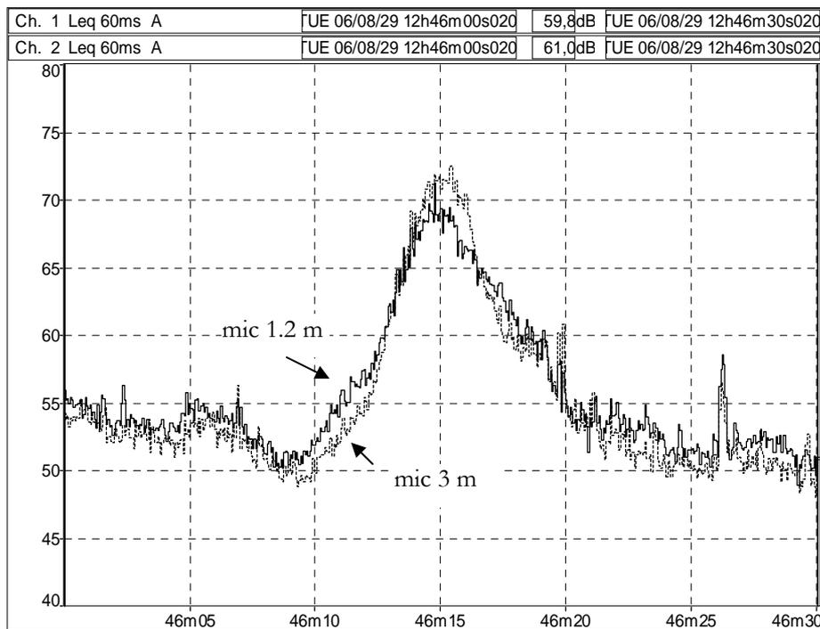
Figure 23 Example of measurement of an accelerating car. On the axes: x-axis time [s], y-axis sound pressure level [dB re 20 μPa].
