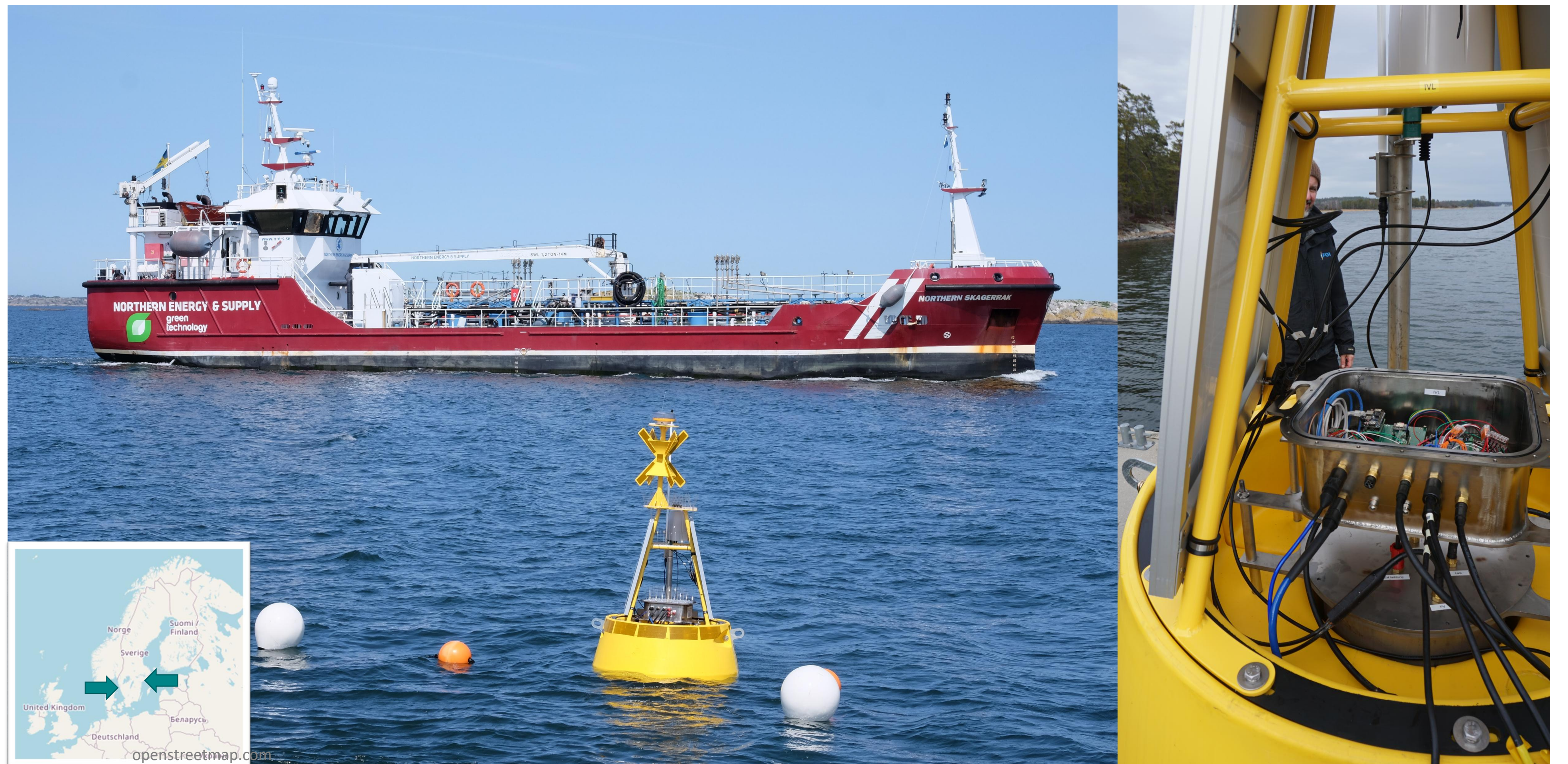
The InciteShip buoys measure ship URN signatures using three cabled hydrophones.
