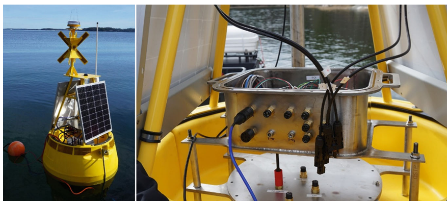
Fig. 2 Photos of the InciteShip system surface buoy (left) and the electronics and battery boxes (right)
