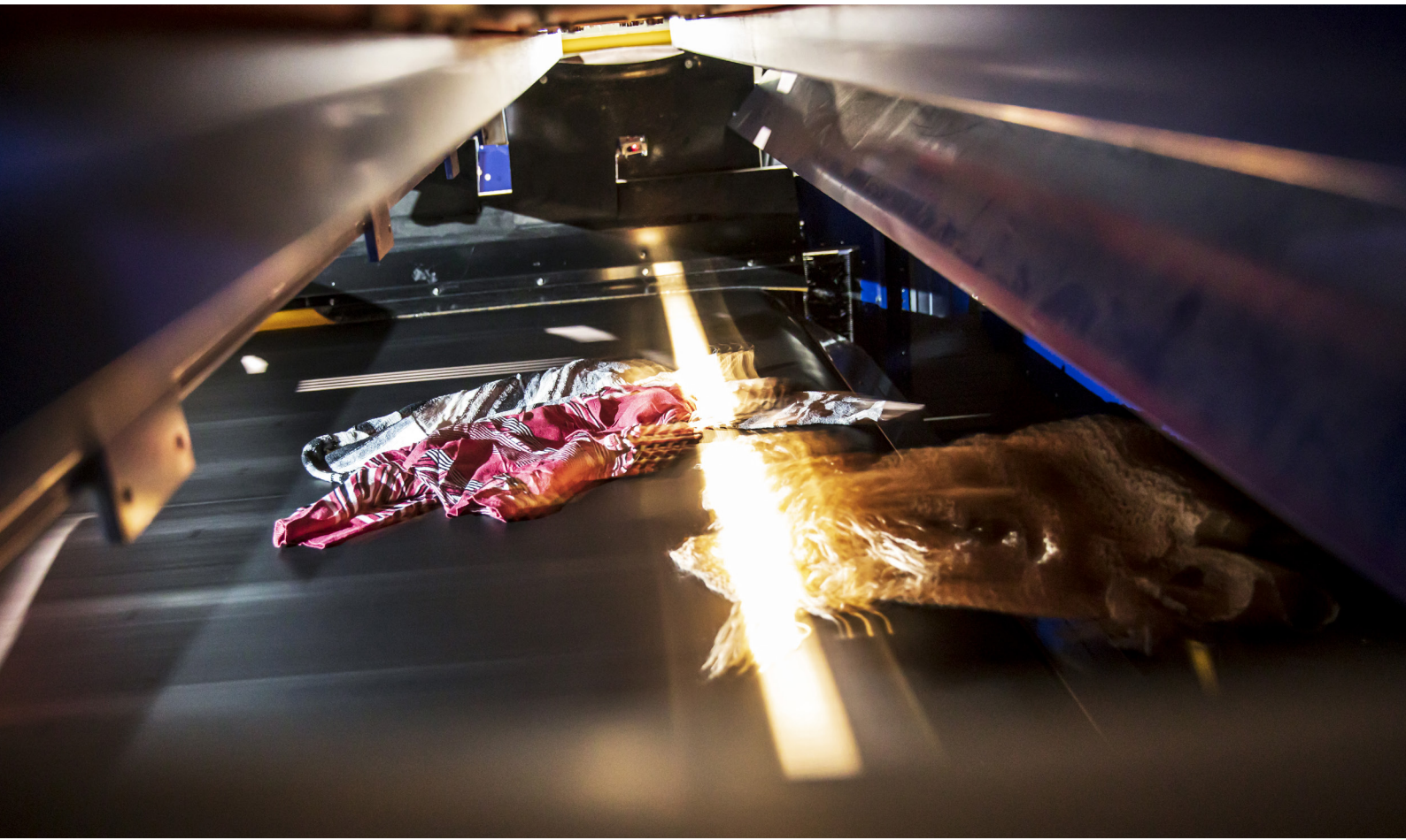
The Siptex facility uses near-infrared and visual spectroscopy to sort mixed textile waste in terms of fibre composition and colour.
