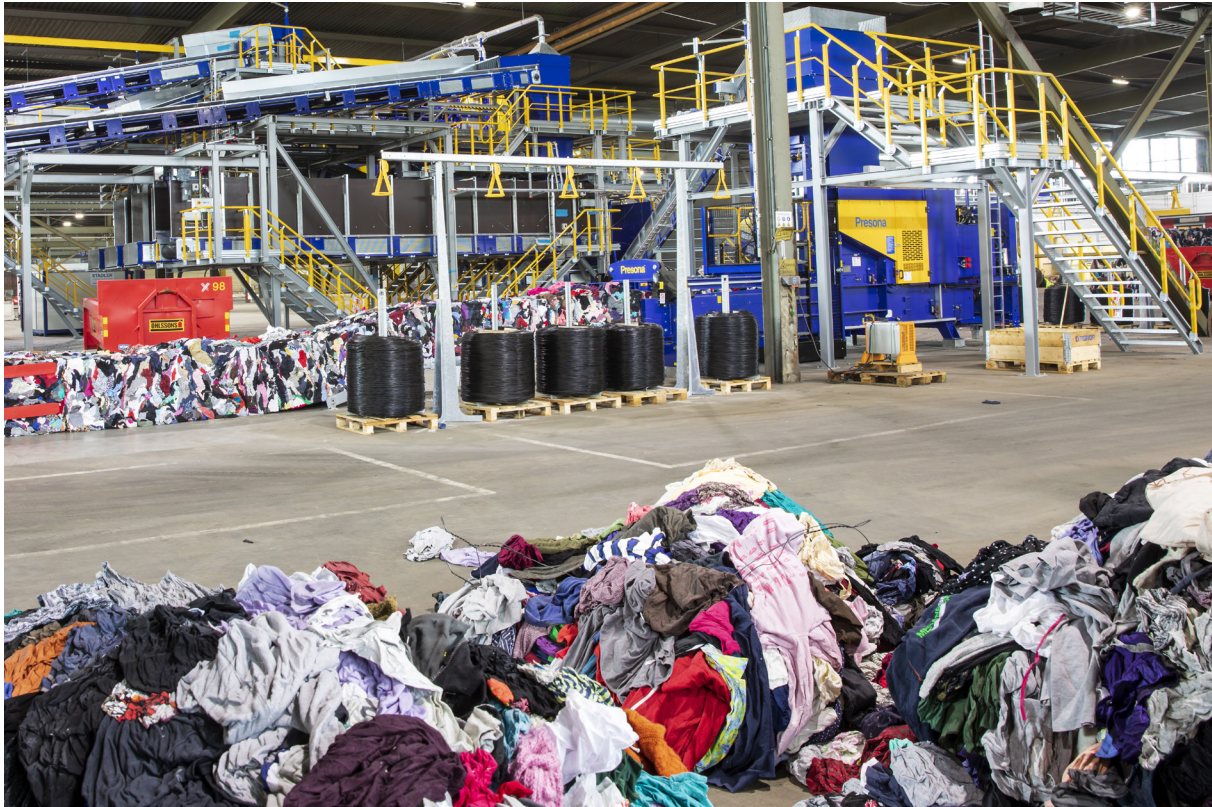
Several challenges remain in textile sorting, for example the need for manual pre-sorting as the Siptex facility cannot handle products such as multi-layer garments and upholstered products.
