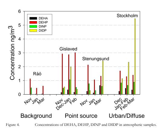
The adipate, DEHA, occurred in lower concentrations compared with the phthalates, which was expected considering the lower consumption level of this substance (Figure 1).
