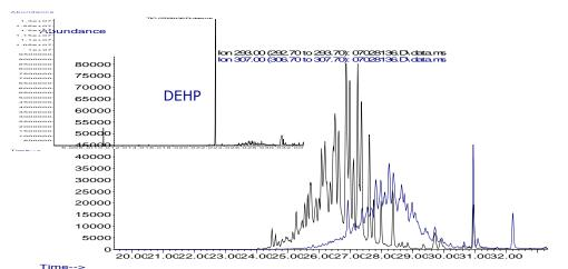
Figure 3. Chromatograms of the iso-phthalates DINP and DIDP and the single substance phthalate DEHP (small picture). Equal amounts give approximately equal areas under the curve hence iso-phthalates are more difficult to distinguish from background noise.
