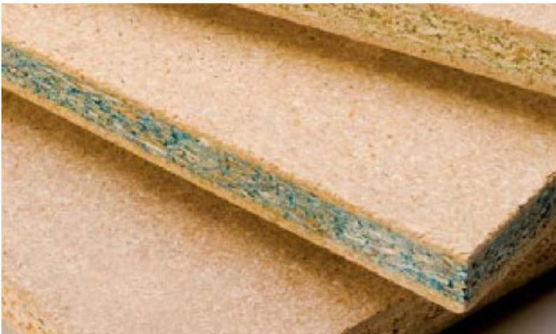
**Figure 1 Particle board made of waste wood**
