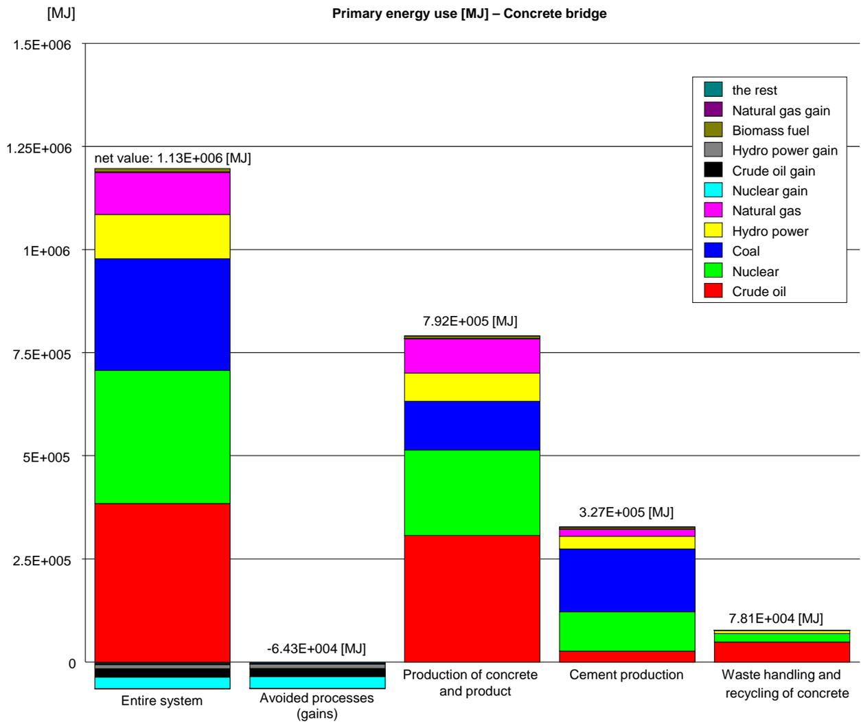
Figure A Primary energy use (excluding waste fuels) for the concrete bridge shown divided into different process groups and for the entire system. The energy net value for the entire system shows the value when avoided energy use has been subtracted.
