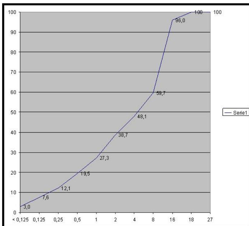
**Figure 4 Example of a particle size distribution for a typical crushed concrete material. The maximum mesh size is here smaller than in a normal crushed concrete fraction. The figure shows the distribution in percent as a function of particle size in mm in a cumulative function.**
