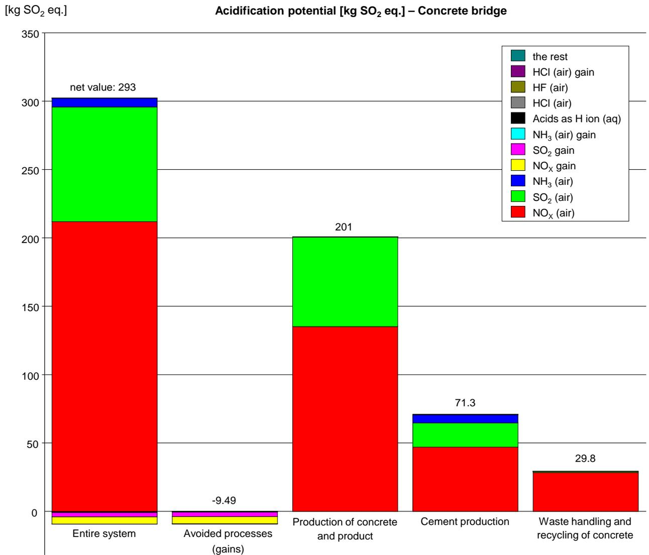
Figure 9 Acidification potential for the concrete bridge shown divided into different process groups and for the entire system. The net value for the entire system shows the value when avoided emissions have been subtracted. The acidification potential is calculated as kg SO<sub>2</sub> equivalents.
