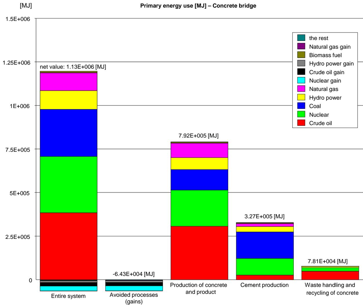
Figure 6 Primary energy use (excluding waste fuels) for the concrete bridge shown divided into different process groups and for the entire system. The energy net value for the entire system shows the value when avoided energy use has been subtracted.
