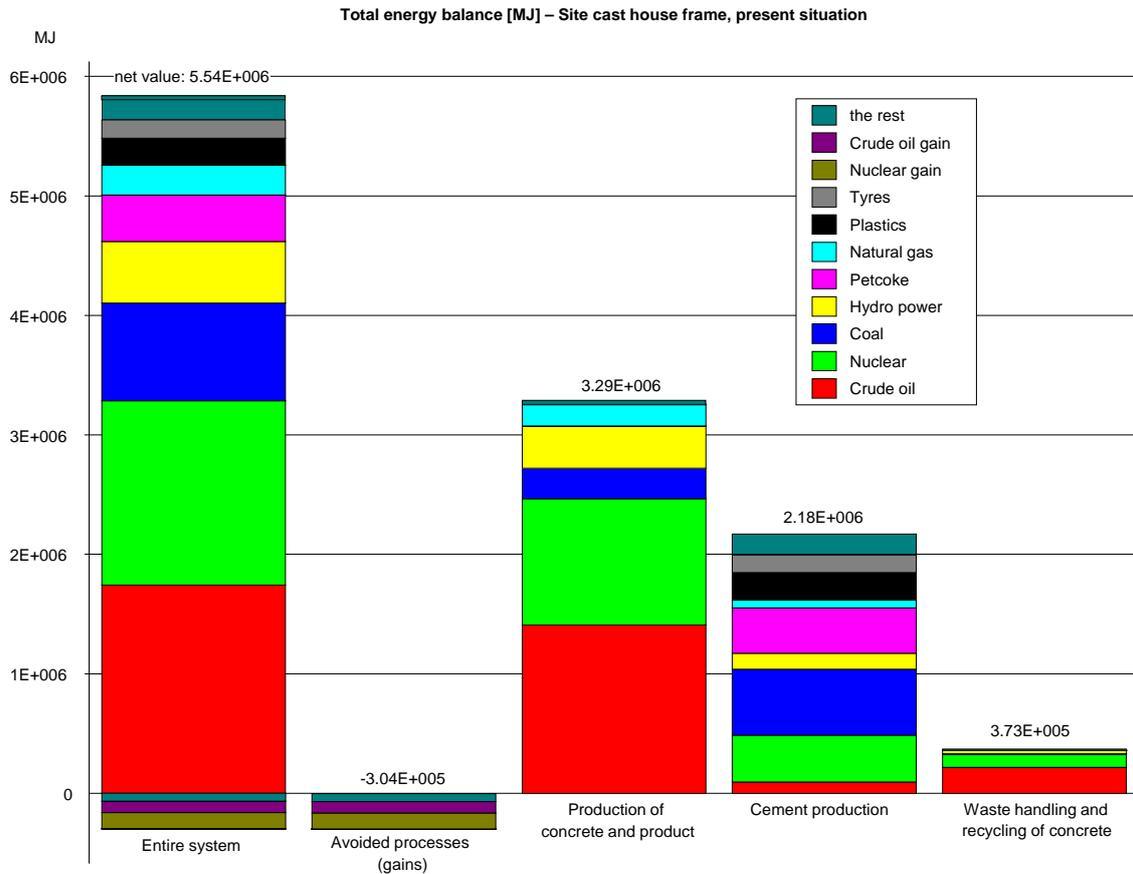
Figure 26 Total energy balance in present production including waste fuels for the site cast house frame shown divided into different process groups and for the entire system. The energy net value for the entire system shows the value when avoided energy use has been subtracted.
