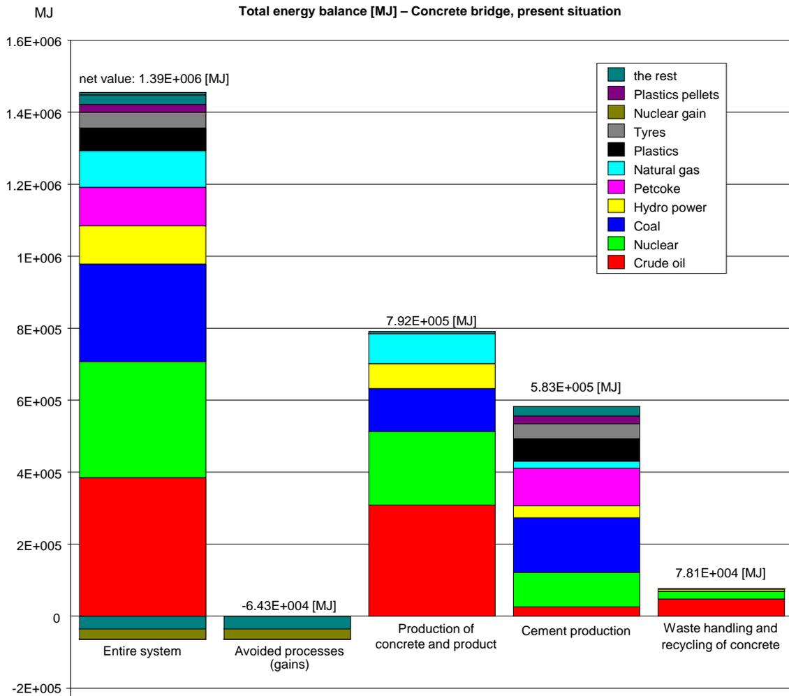
Figure C Total energy balance in present production including waste fuels for the concrete bridge shown divided into different process groups and for the entire system. The energy net value for the entire system shows the value when avoided energy use has been subtracted.
