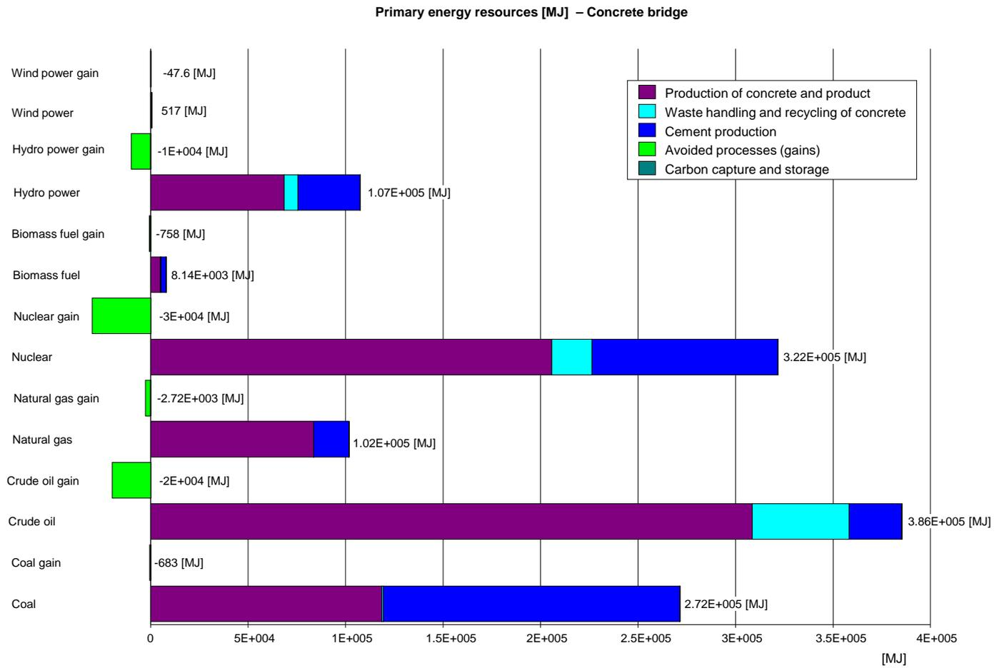
**Figure 7 Primary energy resources (excluding waste fuels) and avoided resource uses (gains) for the concrete bridge. Contributions from the different process groups are shown. The figure includes the entire system.**
