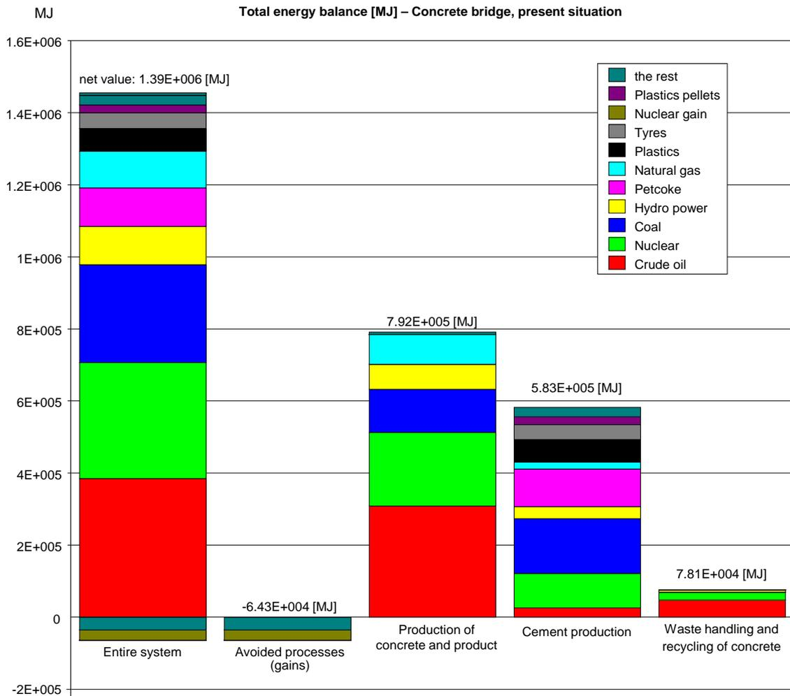
Figure 22 Total energy balance in present production including waste fuels for the concrete bridge shown divided into different process groups and for the entire system. The energy net value for the entire system shows the value when avoided energy use has been subtracted.
