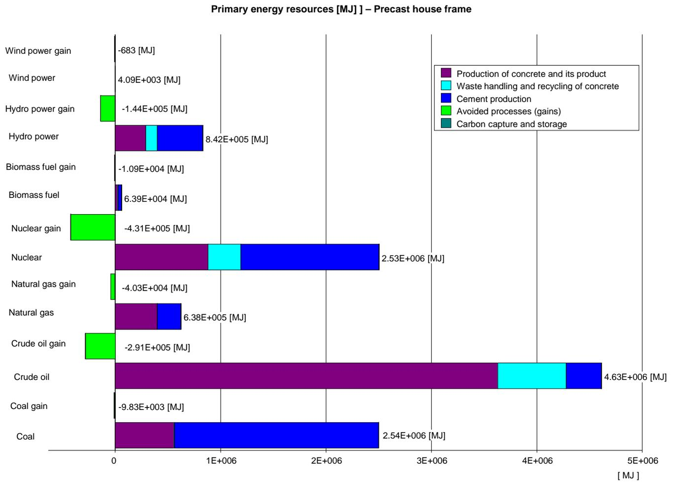
Figure 15 Primary energy resources (excluding waste fuels) and avoided resource uses (gains) for the precast house frame. Contributions from the different process groups are shown. The figure includes the entire system.
