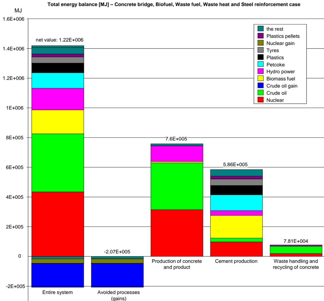
**Figure D** Total energy balance including waste fuels for the concrete bridge shown divided into different process groups and for the entire system. The figure shows the new scenario case with coal replaced with biofuel in the cement kiln, waste fuels as today, increased waste heat recovery and steel reinforcement produced by Swedish EAF. The energy net value for the entire system shows the value when avoided energy use has been subtracted.
