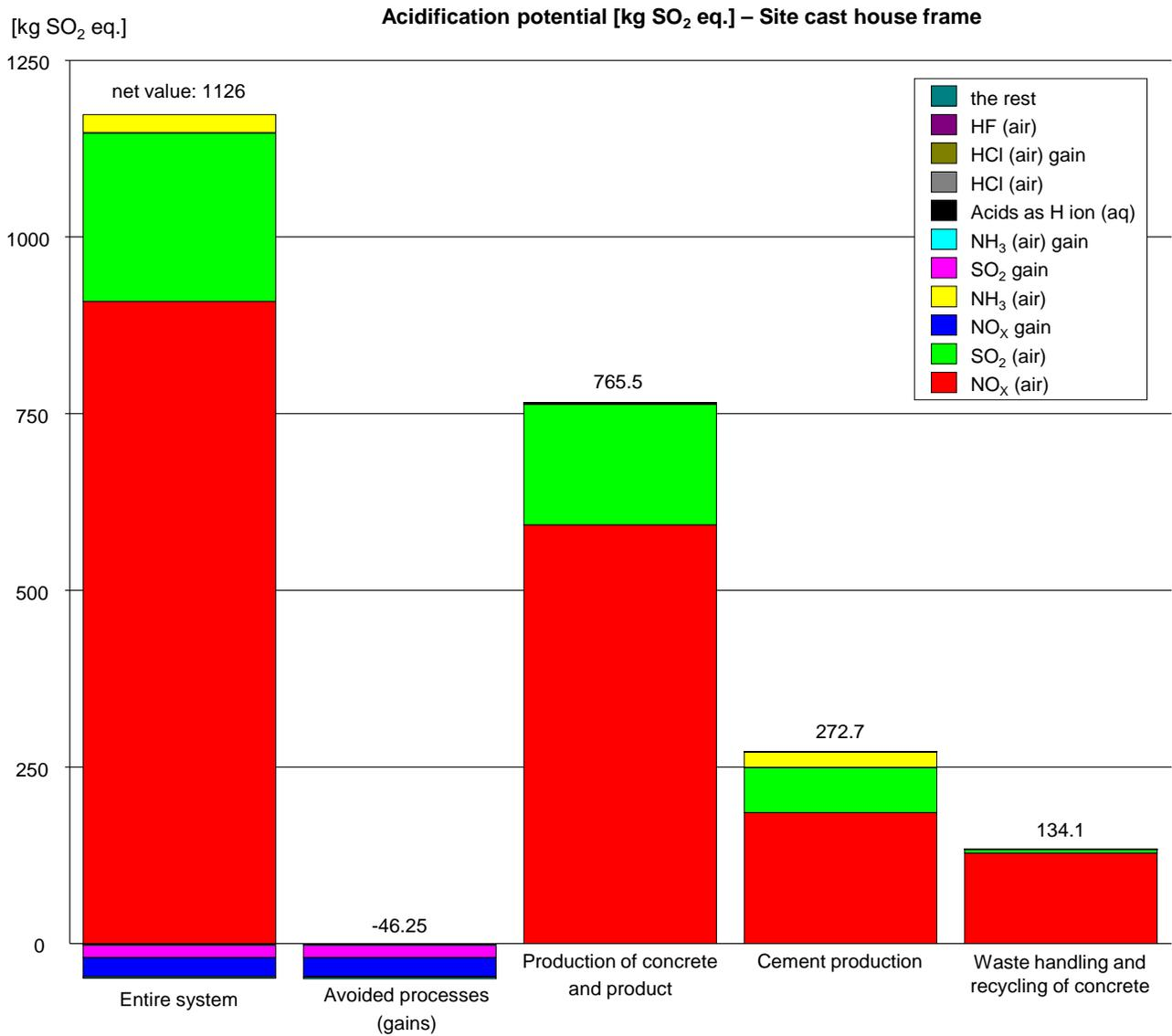
Figure 13 Acidification potential for the site cast house frame shown divided into different process groups and for the entire system. The net value for the entire system shows the value when avoided emissions have been subtracted. The acidification potential is calculated as kg SO<sub>2</sub> equivalents.
