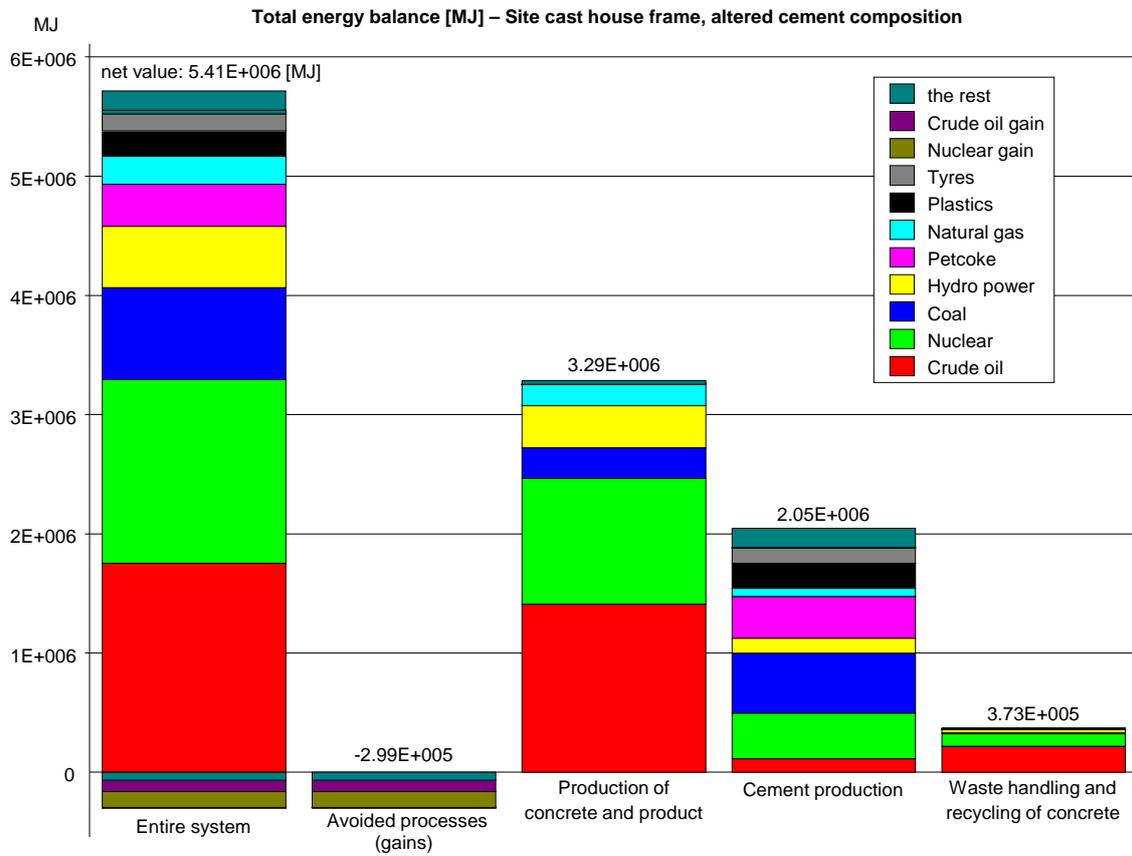
Figure 27 Total energy balance including waste fuels for the site cast house frame produced with an altered cement composition shown divided into different process groups and for the entire system. The energy net value for the entire system shows the value when avoided energy use has been subtracted.
