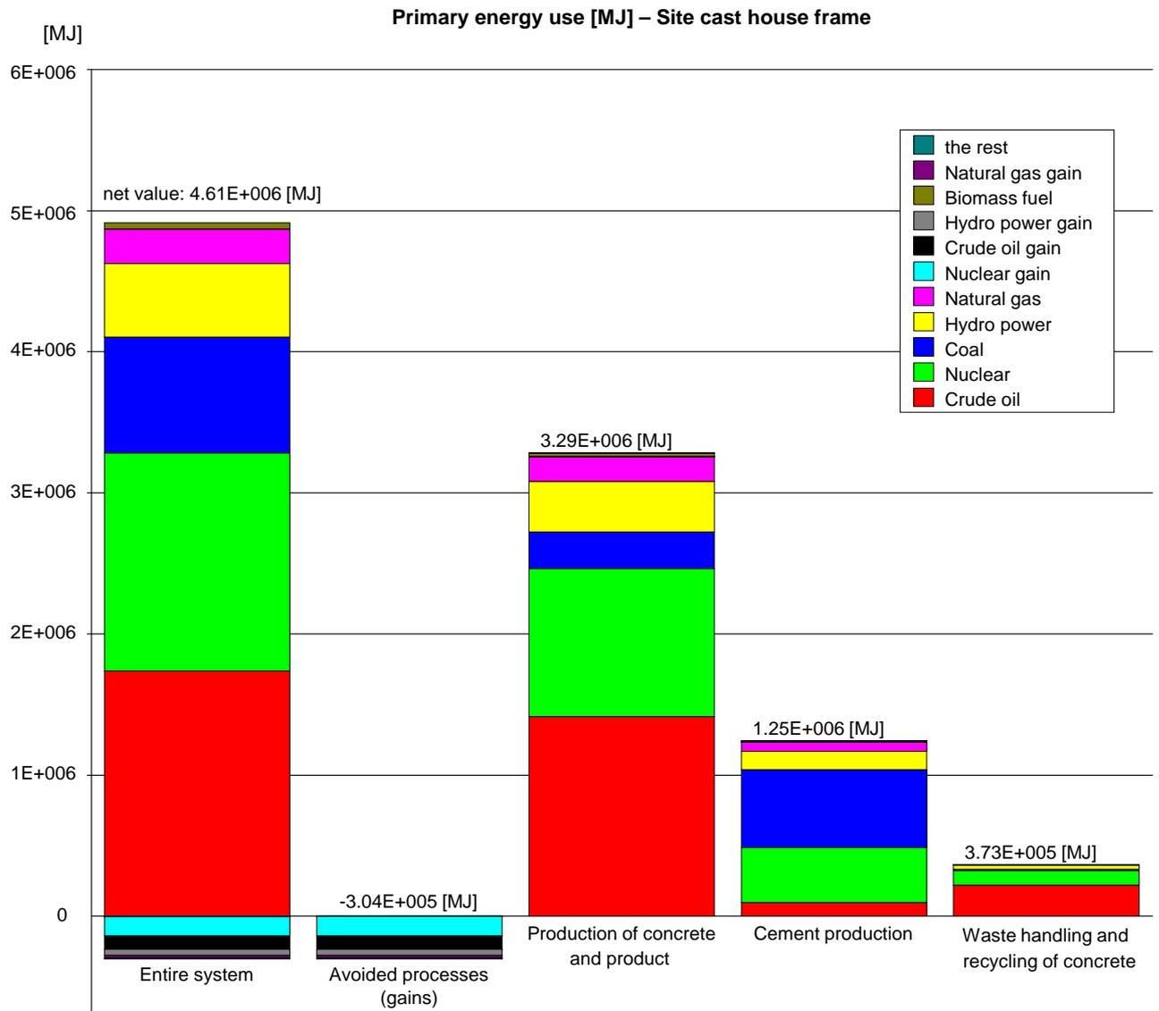
Figure 10 Primary energy use (excluding waste fuels) for the site cast house frame shown divided into different process groups and for the entire system. The energy net value for the entire system shows the value when avoided energy use has been subtracted.
