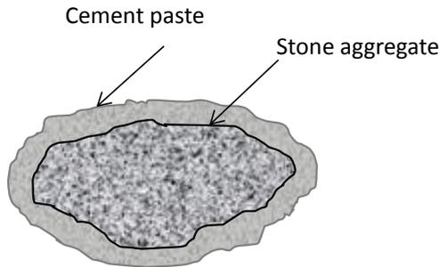
Figure 5 Schematic figure of a crushed concrete aggregate.
