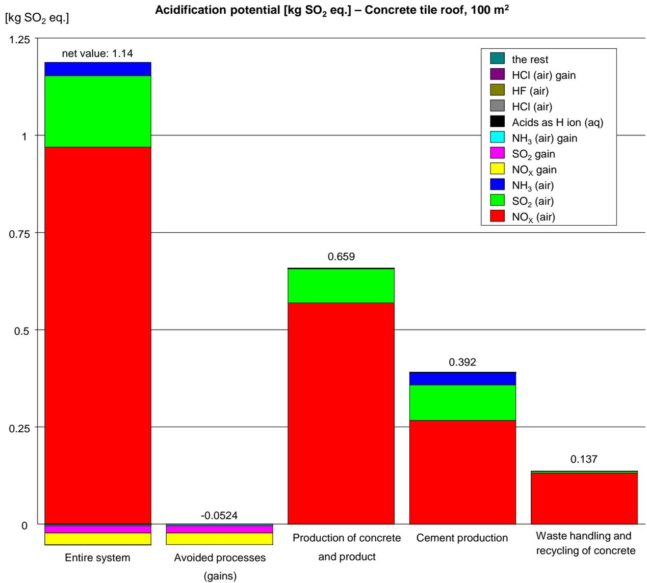
**Figure 21** Acidification potential for 100 m<sup>2</sup> concrete tile roof, shown divided into different process groups and for the entire system. The net value for the entire system shows the value when avoided emissions have been subtracted. The acidification potential is calculated as kg SO<sub>2</sub> equivalents.
