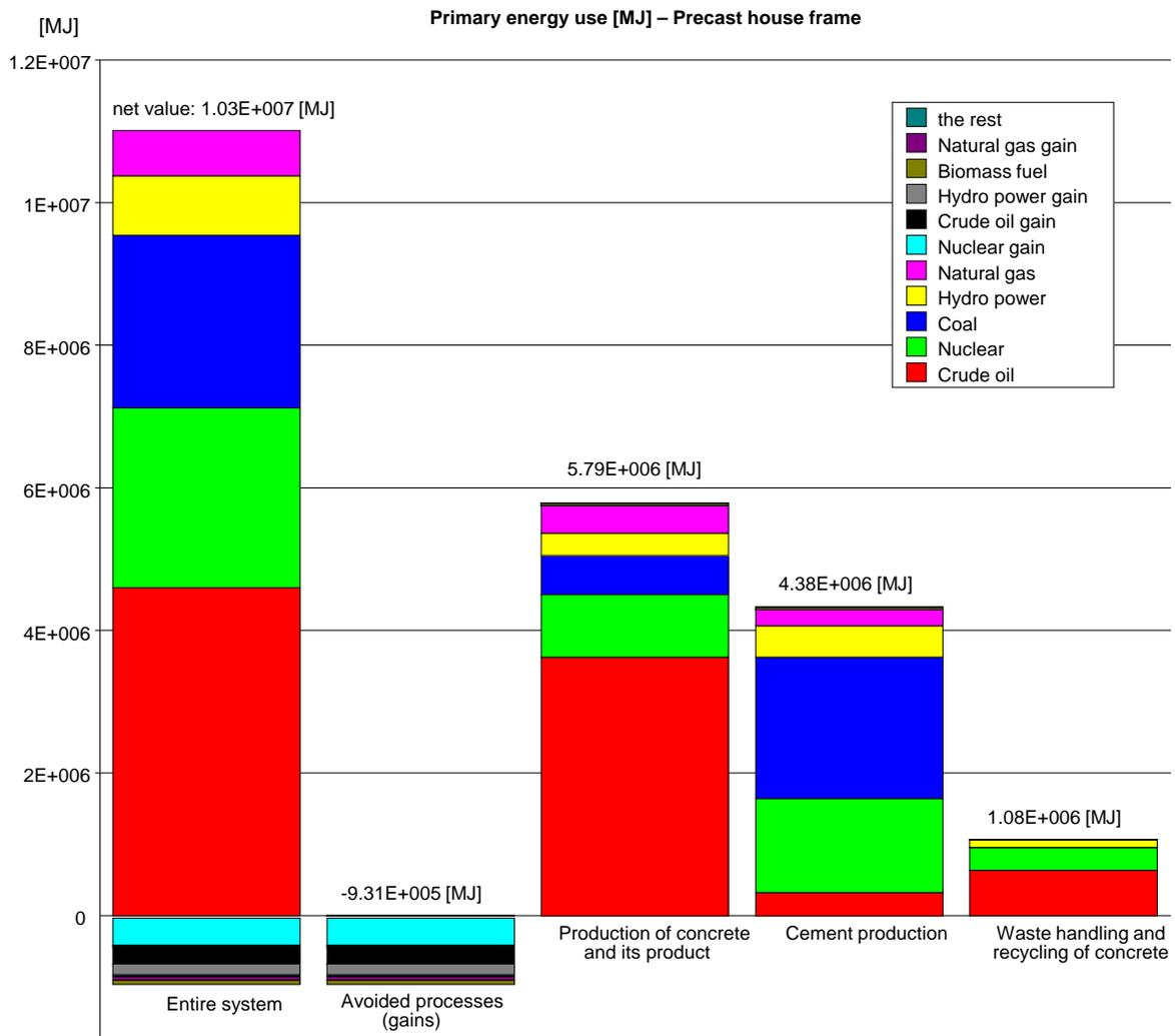
Figure 14 Primary energy use (excluding waste fuels) for the precast house frame shown divided into different process groups and for the entire system. The energy net value for the entire system shows the value when avoided energy use has been subtracted.
