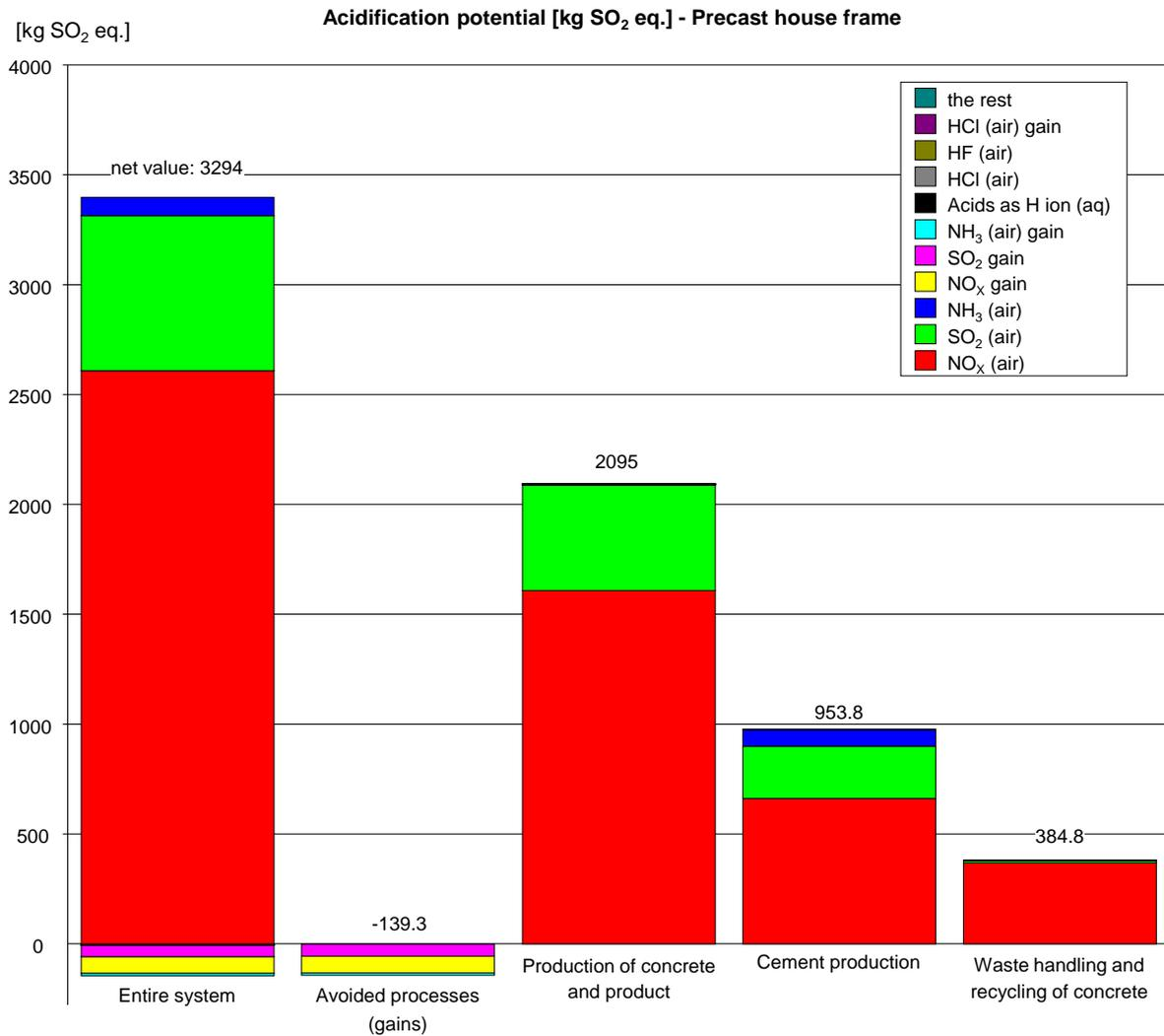
**Figure 17** Acidification potential for the precast house frame shown divided into different process groups and for the entire system. The net value for the entire system shows the value when avoided emissions have been subtracted. The acidification potential is calculated as kg SO<sub>2</sub> equivalents.
