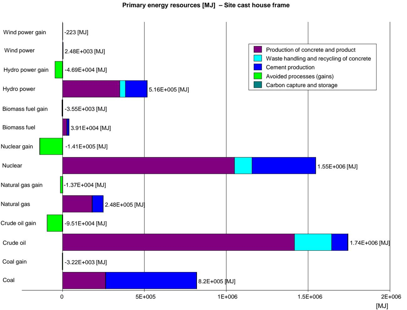
Figure 11 Primary energy resources (excluding waste fuels) and avoided resource uses (gains) for the site cast house frame. Contributions from the different process groups are shown. The figure includes the entire system.
