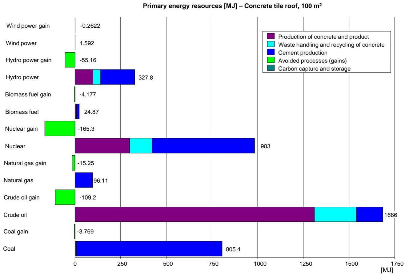
**Figure 19** Primary energy resources (excluding waste fuels) and avoided resource uses (gains) for 100 m<sup>2</sup> concrete tile roof. Contributions from the different process groups are shown. The figure includes the entire system.
