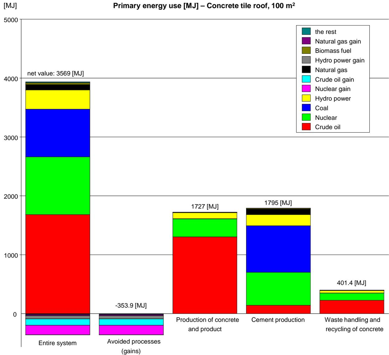
**Figure 18** Primary energy use (excluding waste fuels) for 100 m<sup>2</sup> concrete tile roof. The figure shows the result divided into different process groups and for the entire system. The energy net value for the entire system shows the value when avoided energy use has been subtracted.
