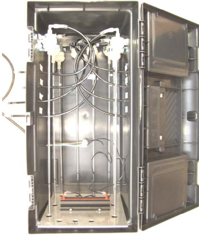
Figure 2. Heated box with 8 denuders and impregnated filters.
