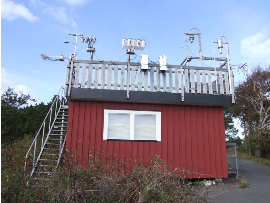
Figure 1. EMEP station at Råö with boxes for \text{NH}_3/\text{NH}_4^+ and \text{HNO}_3/\text{NO}_3^- . The filter packs as well as samplers for \text{PM}_{10} and \text{PM}_{2.5} can also be seen on the photo.
