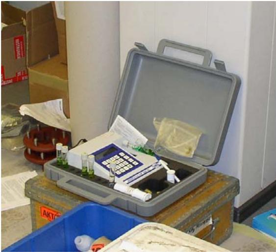
Figure 11. Photometer used for ammonium ion measurements.
