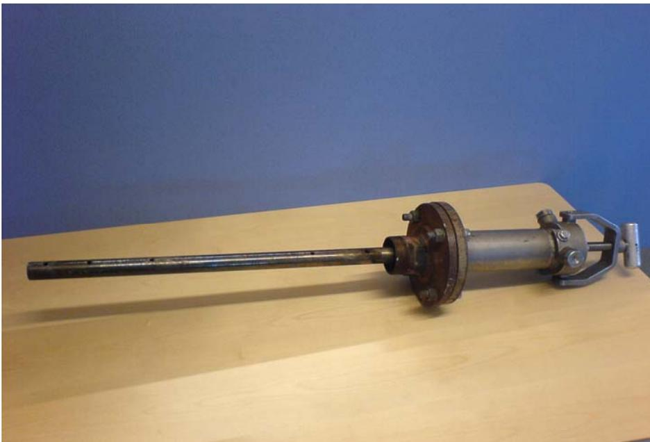
Figure 17. Probe used for gas sampling to the FTIR system and the Horiba instrument.
