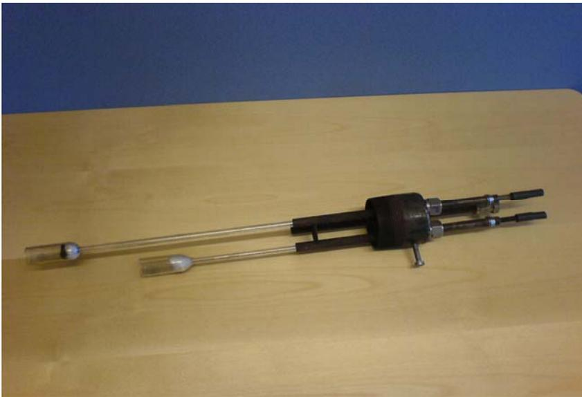
Figure 10. The probe used for wet chemistry sampling.
