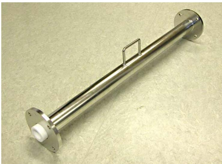
Figure 33. The stainless tube used for the ex-situ tests with the laser system in the lab.
