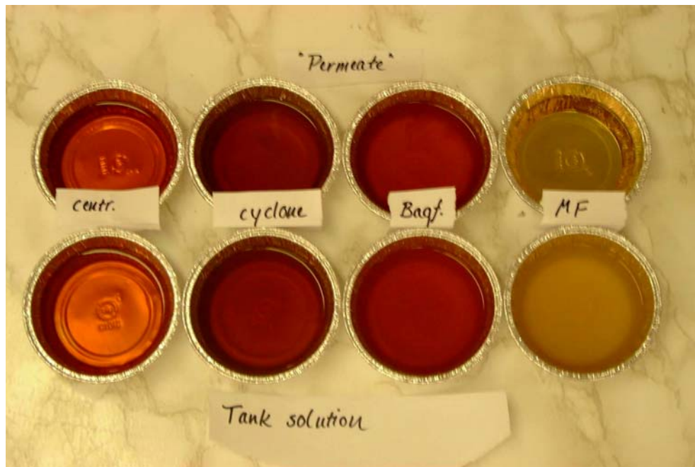
Figure 3.1 Samples from ingoing (tank solution) and outgoing (permeate) solution from each technique tested. From right; micro filtration, bag filter, hydrocyclone and centrifugation. The bath solution was changed between running of the hydrocyclone and the centrifuge. There is a visual difference in turbidity between the tank solution and permeate on the micro filtration but not on the other samples. There is also a difference in turbidity between the centrifugation and the other samples.
