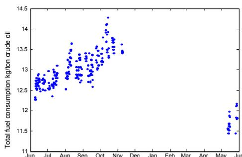
Figure 7 Total relative fuel consumption, variation in time (chemical cleaning during winter stop).
