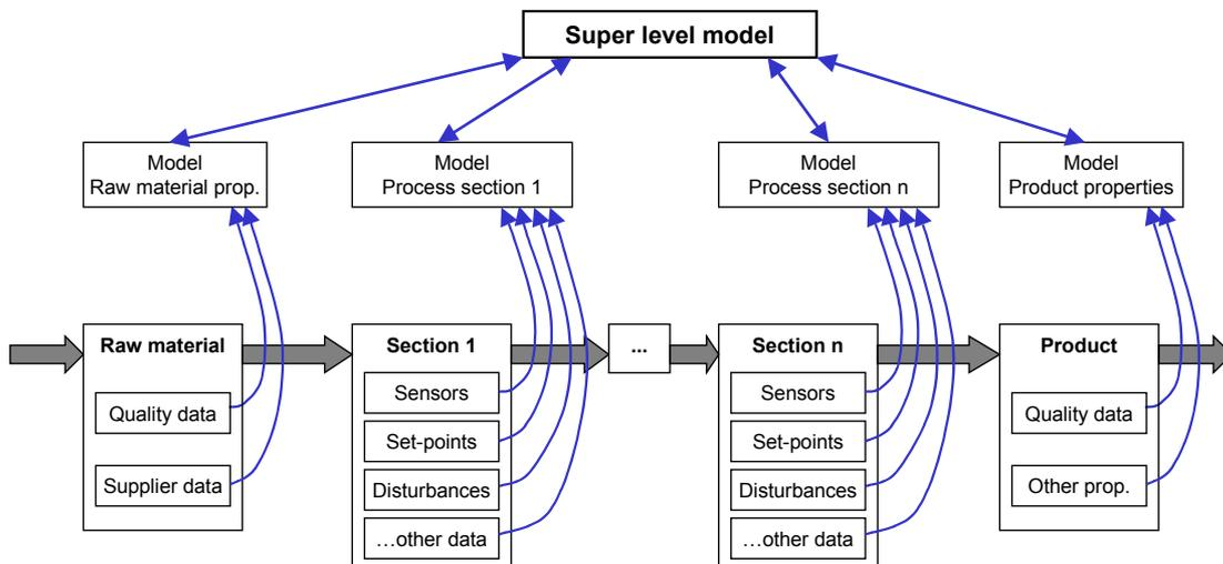
Figure 1. Schematic picture of a multi-block model applied to a multi-step process.
