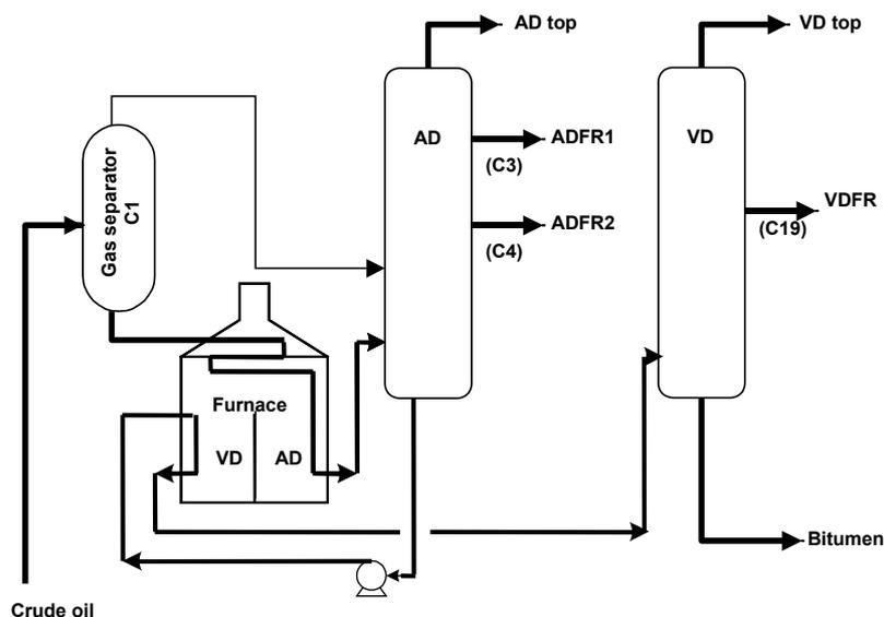
Figure 2 Simplified outline of the distillation process at Nynäs Refining AB. The initial products are the fractions ADTOP, ADFR1, ADFR2, VDTOP, VDFR and bitumen. Mixing of some of these products to form new products also occur.
