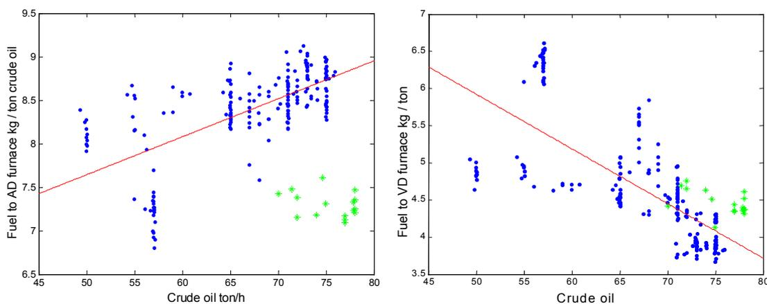
Figure 8 Relation between relative fuel consumption and crude oil feed rate. Left: AD furnace. Right: VD furnace. Before chemical cleaning, blue dots and linear regression, after cleaning, green stars.
