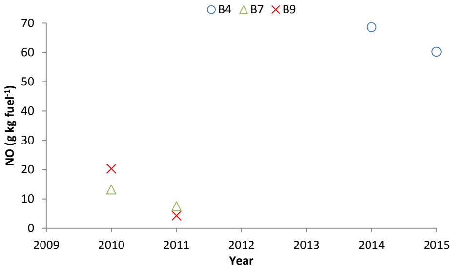
Figure 10 EF_{NO} of buses that have been tested at multiple occasions, excluding buses where there has been a fuel switch and where the changes were not statistically significant.
